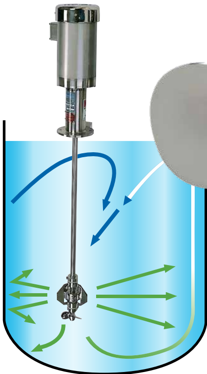
◀ Flow pattern: Blue arrows = flow into the mixing head Green arrows = expulsion from the mixing head
